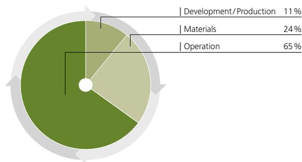
The energy consumed while an elevator is in service (operation phase) accounts for two-thirds of its environmental impact.
